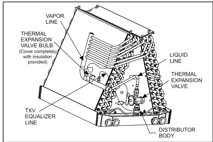
**FIGURE 10:** Thermal Expansion Valve (TXV)
