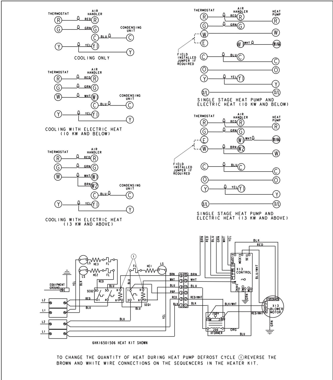
FIGURE 17: Typical Wiring Diagram - ECM
