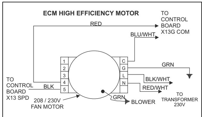
FIGURE 14: Blower Speed Connections
