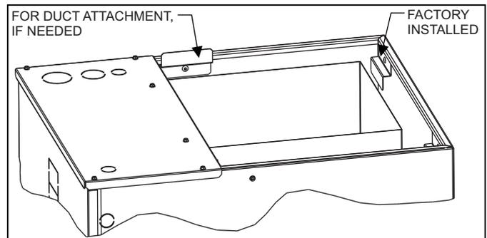
**FIGURE 8:** Duct Attachment
