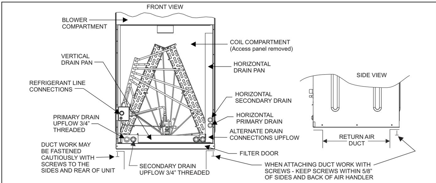
**FIGURE 1:** Return Duct Attachment & Component Location
