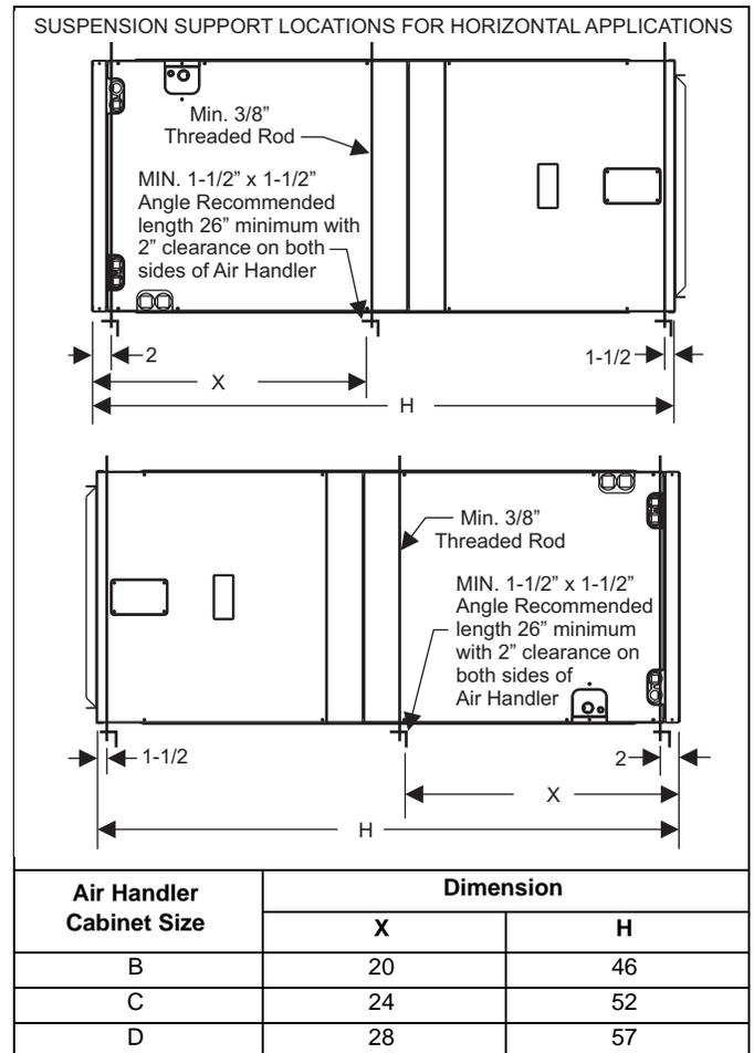
**FIGURE 7:** Horizontal Suspension
