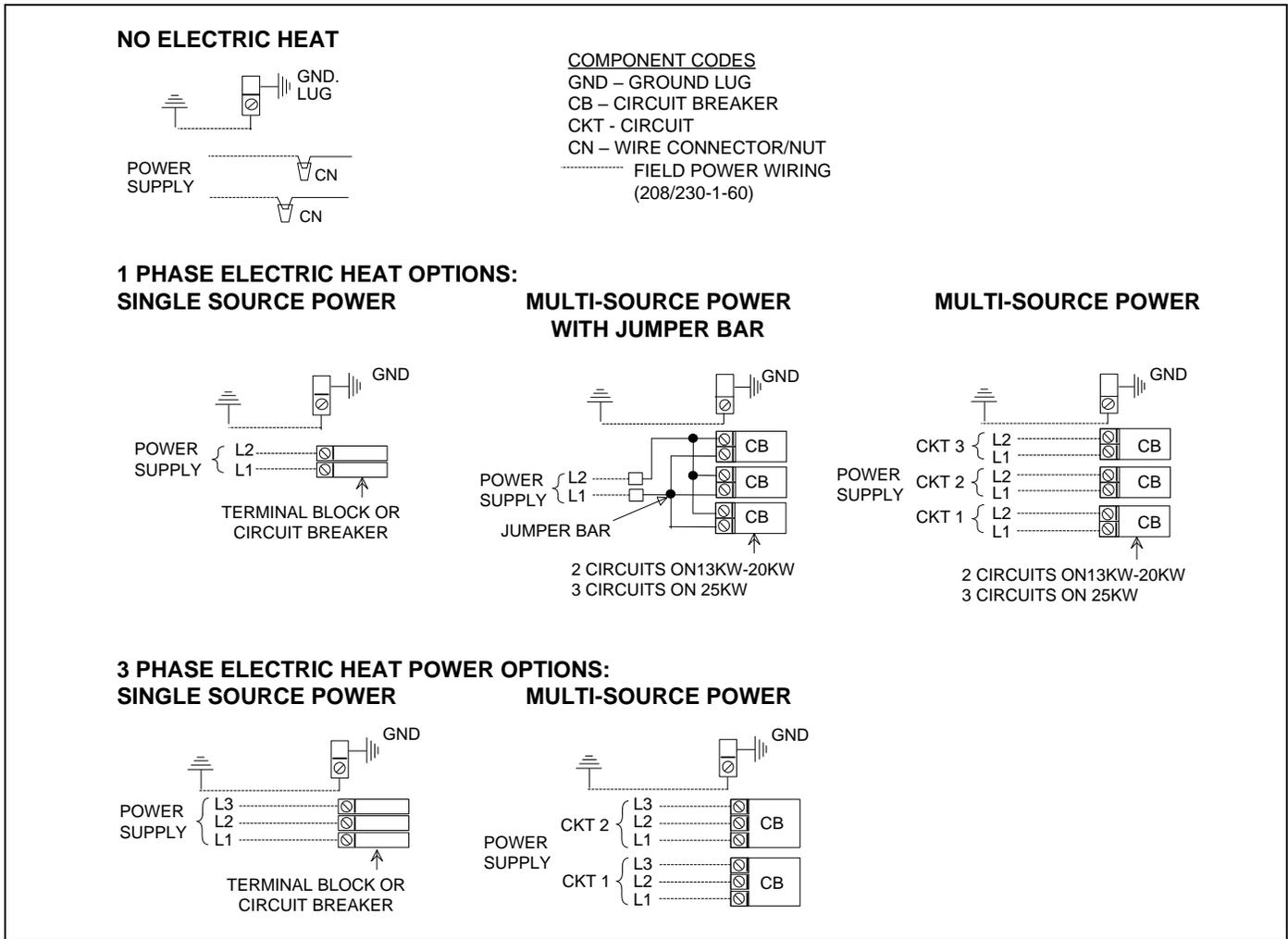
FIGURE 13: Line Power Connections
