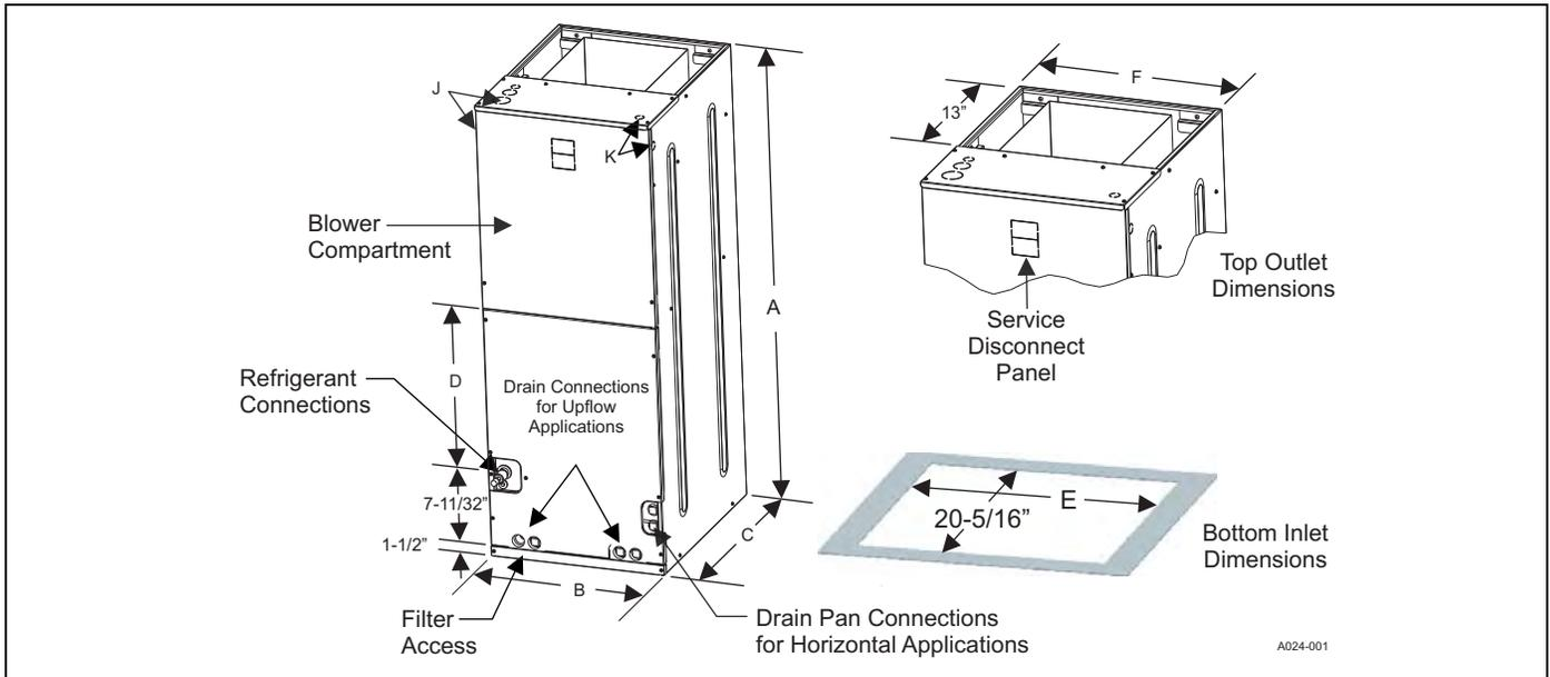
**FIGURE 2:** Dimensions & Duct Connection Dimensions
