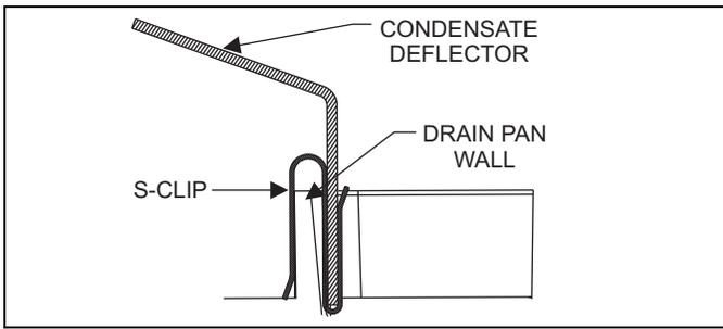
**FIGURE 6:** S-Clip Installation
