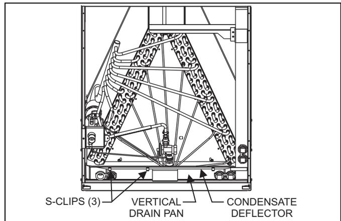
FIGURE 4: Condensate Deflector on Vertical Drain Pan
