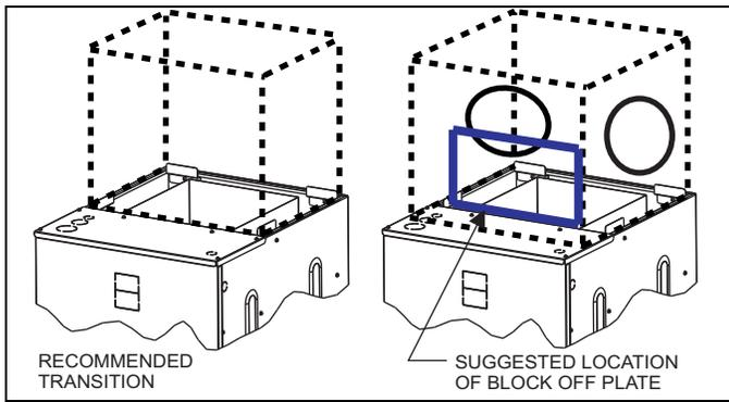
**FIGURE 9:** Ductwork Transition
