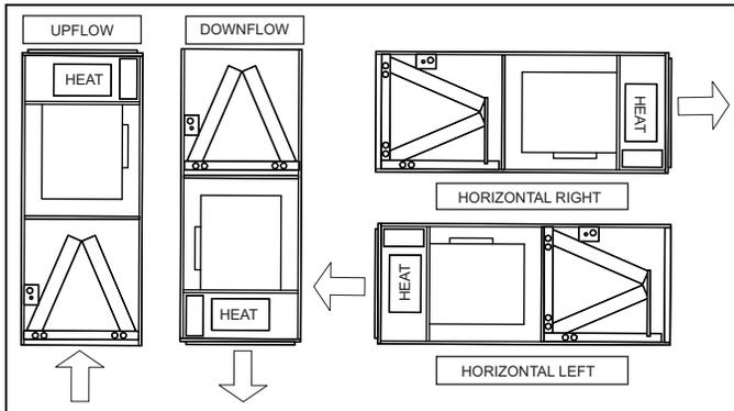
FIGURE 3: Typical Installation
