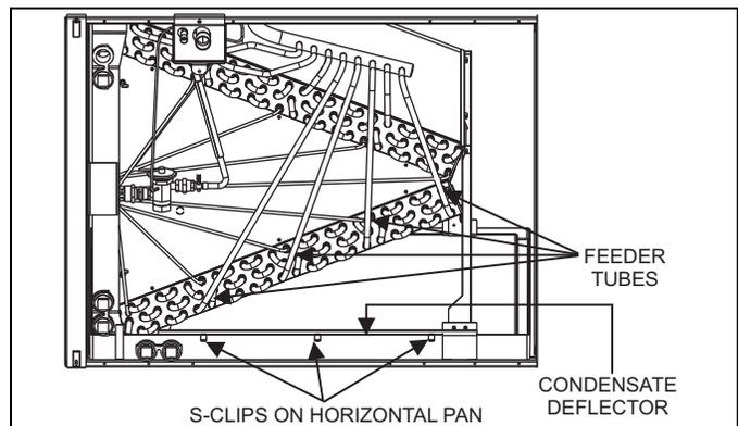
FIGURE 5: Condensate Deflector on Horizontal Drain Pan Edge
