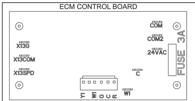
FIGURE 12: Blower Delay Control Board
